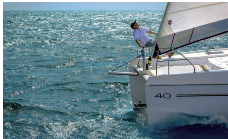
↑ The Leopard 40 shows an overall balance which, thanks to the fineness of the hulls and good bridgedeck clearance (78cm), allows it to remain comfortable and perform well in a choppy sea, even upwind.
