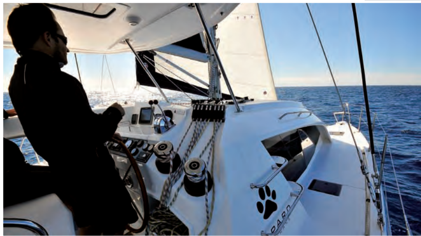
The helm station is good, and the amount of kit here doesn't impinge on sail handling, thanks to the assistance of the electric winch. Taking in a reef (with the continuous reefing lines) is easy, as is furling the genoa. Visibility is good, and the feel of the helm is direct thanks to the mechanical linkages.
