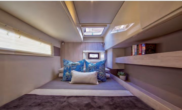
Ventilation, storage and large portlights for a good exterior view. The aft cabins are comfortable and the headlinings cleverly secured with clips, making them removable
