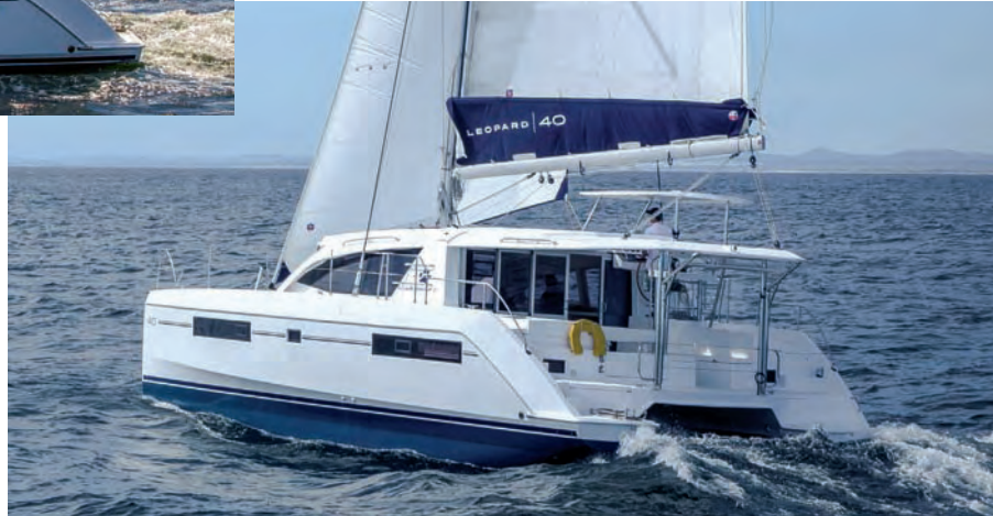
↓ The forward third of the hull is fairly narrow, increasing as it comes aft to the very load-bearing shape of the aft third, allowing nice performance under sail.
