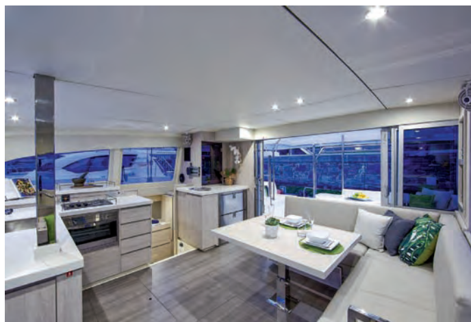
↑ A successful layout in the nacelle. The practical L-shaped galley, very effective fridges, a functional and understandable electric panel and a large dining area to seat 6 to 8 people round a table which transforms into a bunk when under way. The new style of light oak is a clean break with the cherry cabinetry of the previous generation
