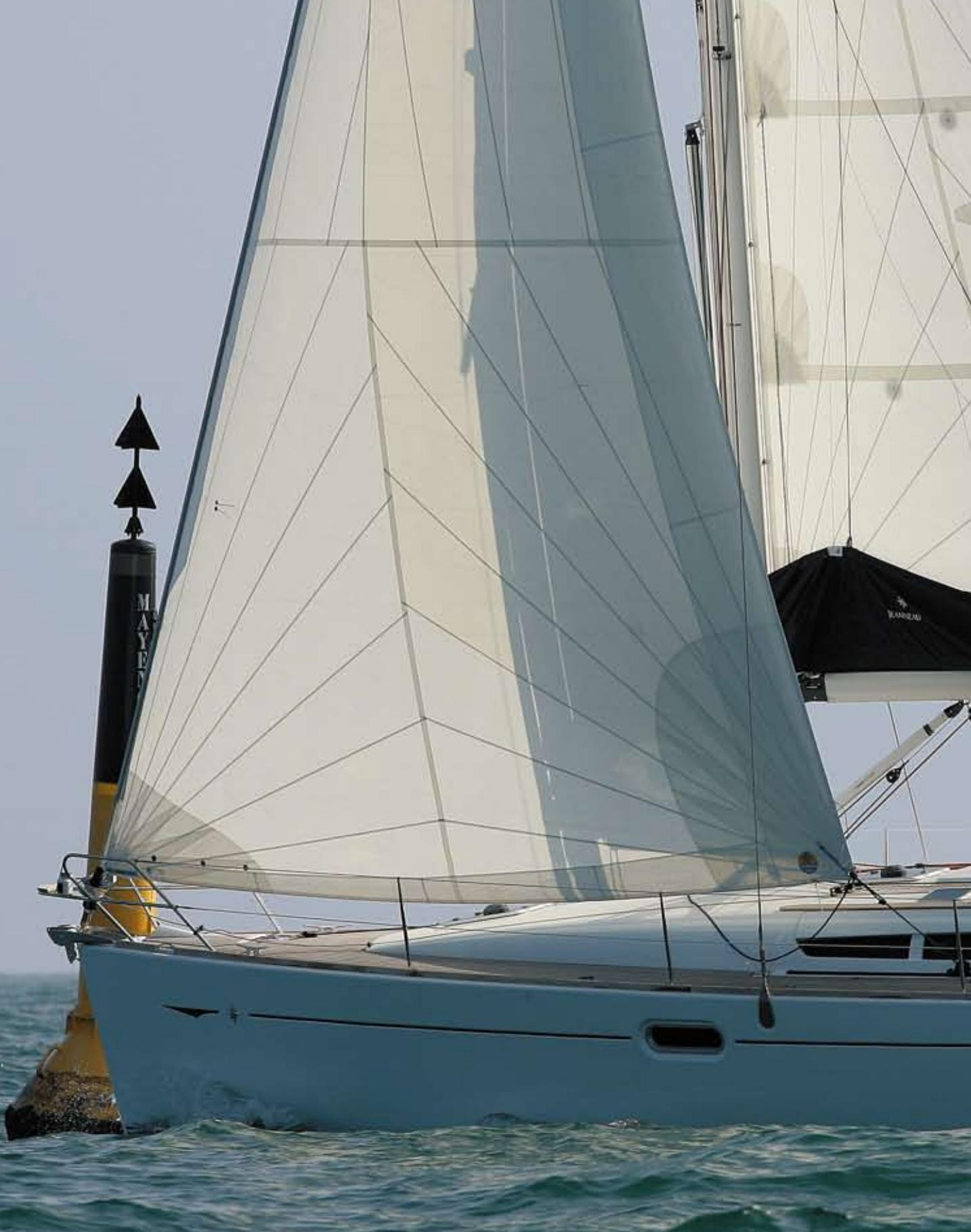
The Performance version of the Sun Odyssey 42i is designed for even more power and speed, fitted with Prestige series sails, tri-radial cut in Mylar/Taffeta, a taller mast, twin groove furler, a folding feathering propeller and more, allowing you to go faster while enjoying the same comfort offered on the standard version.
