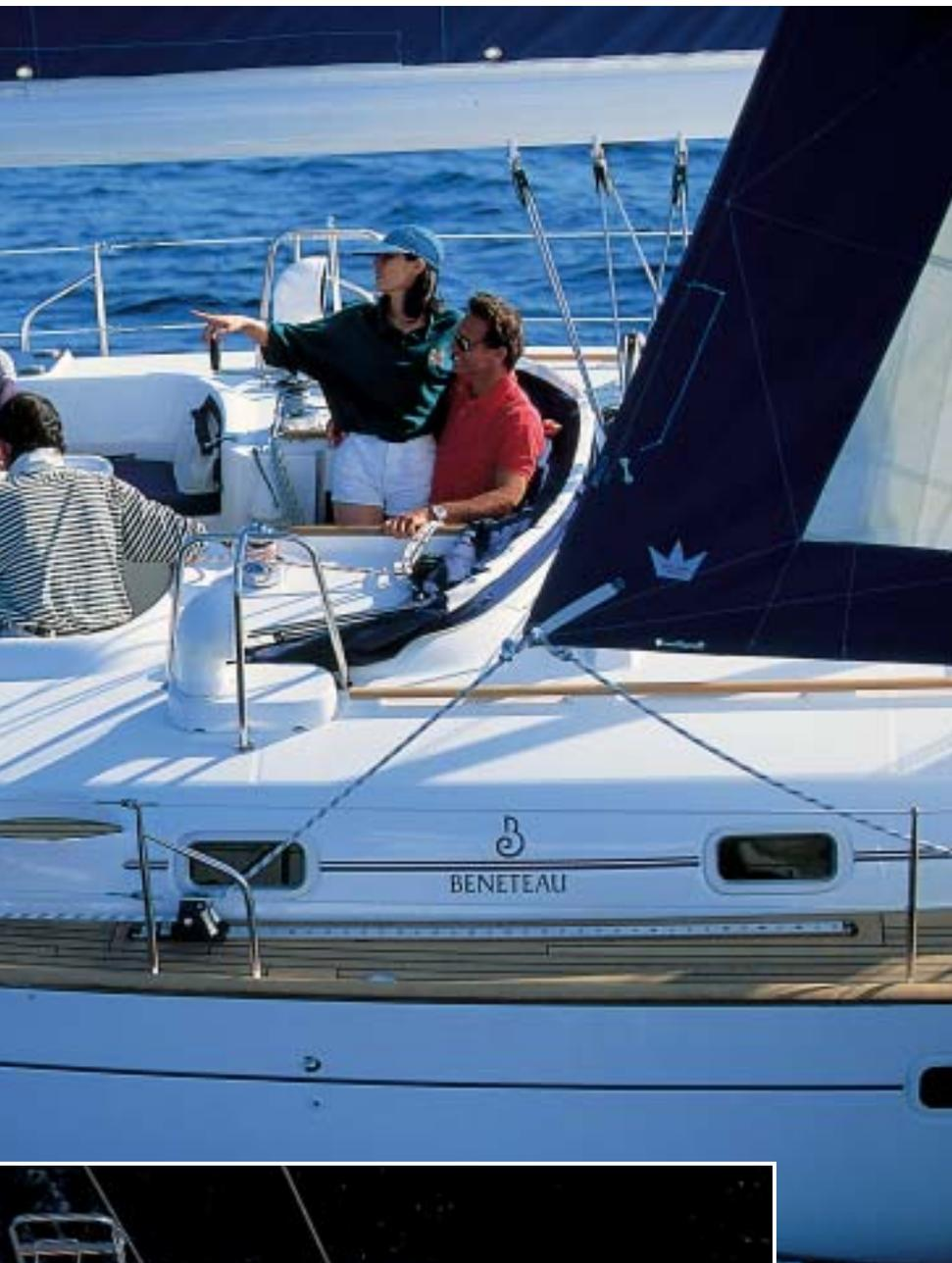
*The deck layout on the Beneteau 50 is state of the art : wide sidedecks, a teak covered bulwark and judiciously located hatches ensure easy and safe circulation on deck.*
