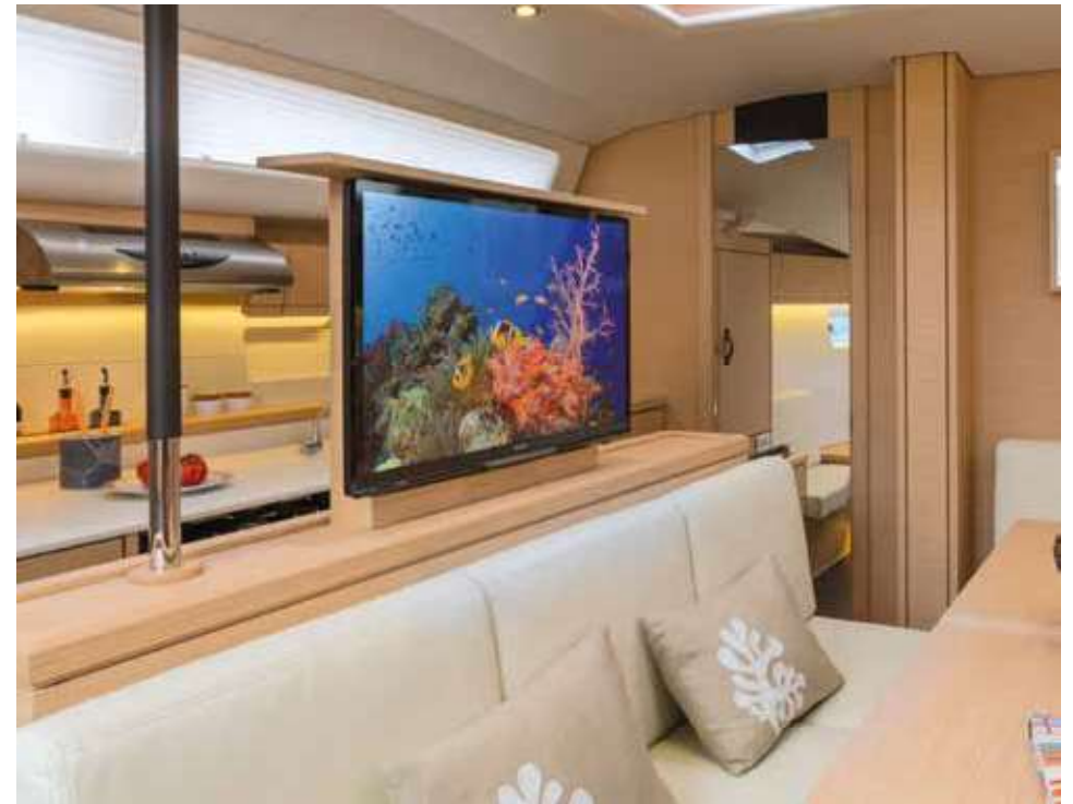
Lifting TV integrated into sofa backrest / Ecran TV escamotable derrière le sofa
