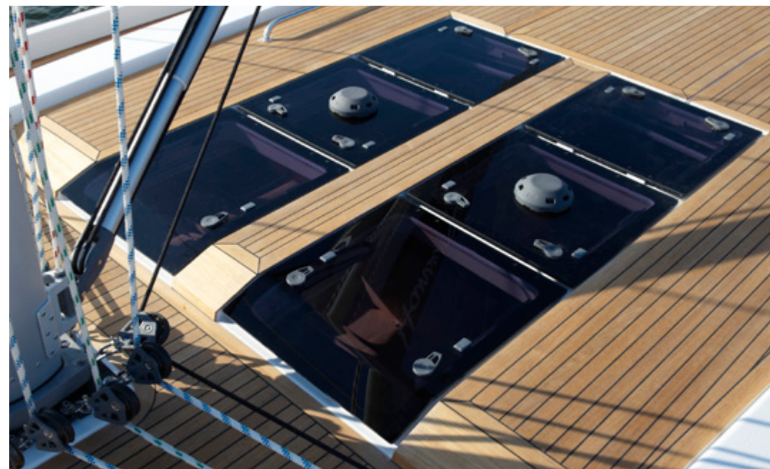
3 Elegantly designed and openable flush hatches above the saloon for lighting and ventilation.
