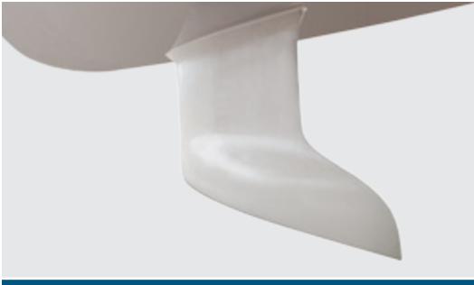
Shallow draft L-shape-keel (2.25 m), cast iron
