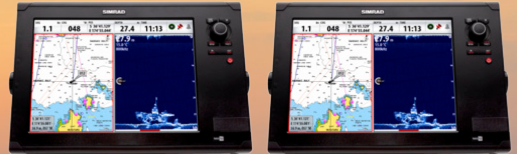
2 SIMRAD NSS 12 touch screen GPS chart plotter with AIS overlay, engine information incl. windtransducer one at each helm position
