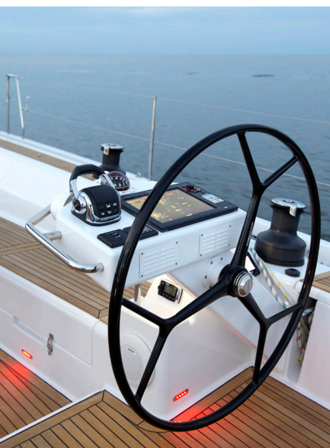
2 Centre: solid steering pedestal with throttle, compass and Simrad NSS 12 touch screen GPS chart plotter.
