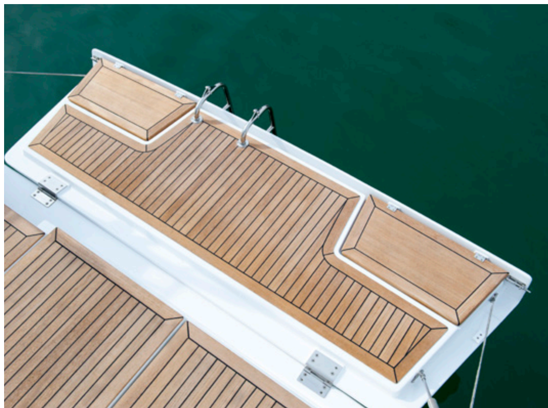
5 A terrace on the sea: manual opening bathing platform with ladder and folding helm seats.
