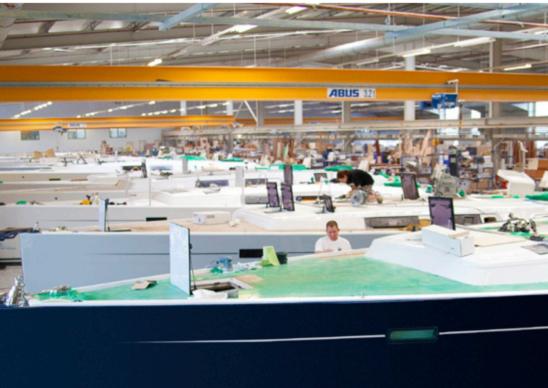
3 Series production of yachts on assembly lines with calculated cycle times - good value with high quality.
