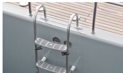
Stainless steel removable ladder to rail gate exit
