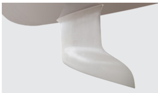
Shallow draft L-shape keel (1.82 m), cast iron
