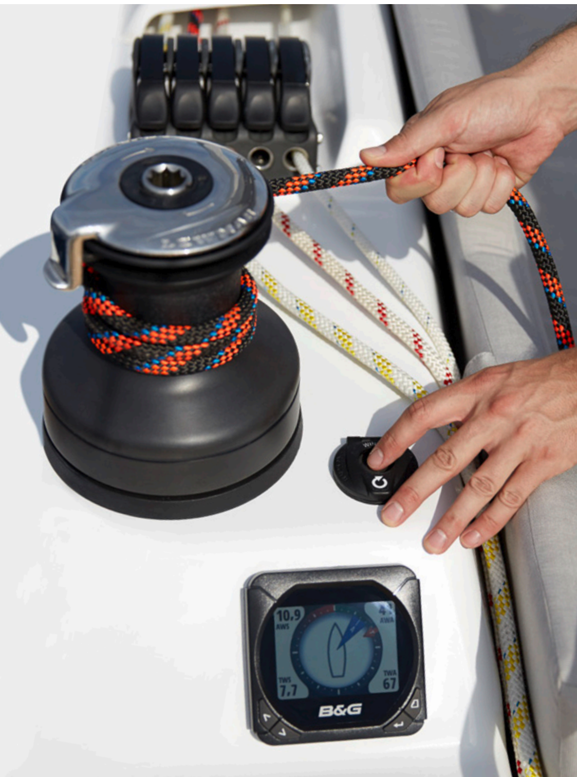
2 Command centre: halyards, sheets and reef lines running to helmsman position.
