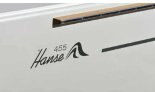
Solid teak and stainless steel rub rail hull protection
