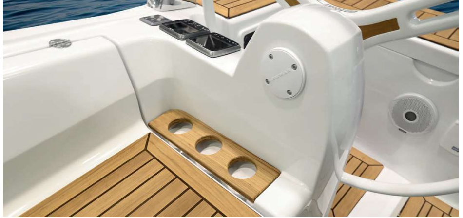
Teak cupholders near at hand for the helmman as well as the crew seated around the cockpit table.
