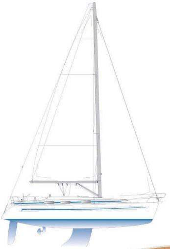
Length overall 37'5" Length hull 36' Length waterline 30'10" Beam 11'10" Draught (standard) 5′1″ Deep lead (option) 6′5″ Displacement 12,100 lbs. 3,300 lbs. Ballast 2 Water tanks 80 gal. Diesel Tank 40 gal. Furling mainsail 290 sq. ft. Battened mainsail 335 sq. ft. 320 sq. ft. 50'6" Ht. of mast above waterline
