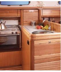
Large galley with gimbaled two burner propane stove with oven and 12 Volt refrigeration
