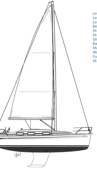
Length overall 31' Length hull 30' Length waterline 27'1" 10'9" Beam 4'7" Draft standard Draft (deep option) 6'1" Displacement 9,240 lbs. Ballast 2,200 lbs. Mainsail & genoa 555 sq. ft. (appx.) Water tank 40 gal. (appx.) Fuel tank 25 gal. (appx.) 46'3" Ht. of mast above waterline
